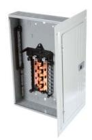
SIEMENS LOW VOLTAGE RISER LOAD CENTER. MAIN LUG WITH 16 1-INCH SPACES ALLOWING MAX 32 CIRCUITS. 1-PHASE 3-WIRE SYSTEM RATED 120/240V (125A) 100KA INTERRUPT. SPECIAL FEATURES: COPPER BUS, INTERCHANGEABLE MAIN, GRAY TRIM.
