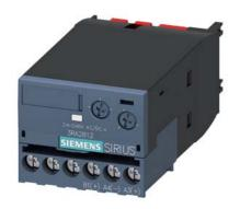
Electronic timing relay OFF delay with control signal and semiconductor output 24...240 V AC/DC Time range 0.05...100 s can be snapped on at the front for contactors 3RT2 S00/S0 and auxiliary contactor 3RH2 S00 Screw terminal Varistor for attenuation of the contactor coil integrated
