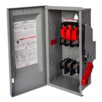
Siemens Low Voltage Circuit Protection Heavy Duty Safety Switches. Type: ENCLOSED, SAFETY SWITCH Std: UL V. Rating: 600V A. Rating: 200A Wattage: 4W No. Of Poles: 3P F. Rating: 60Hz Action: SINGLE THROW Material: STEEL Enclosure: TYPE 1. 2-3 point mounting holes. O. Cycles: 8000 O. Temperature: (-20F-120F) AMBIENT TEMPERATURE Environmental Conditions: INDOOR
