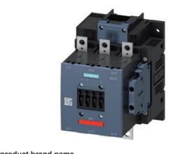
Power contactor, AC-3 150 A, 75 kW / 400 V AC (50-60 Hz) / DC operation UC 110-127 V Auxiliary contacts 2 NO + 2 NC lateral, permanently mounted 3-pole, Size S6 Busbar connections Drive: conventional
