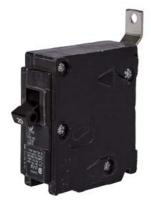
Siemens Low Voltage Molded Case Circuit Breakers Special Application Panelboard Mtg 240V Breakers - HD Ltng 1-pole TM BL 10KAIC 120VAC are Circuit Protection Molded Case Circuit Breakers. Type: BL Special Features: High-Intensity Discharge Application: Electrical Distribution Standard: UL 489 Voltage Rating: 120V Amperage Rating: 20A Trip Range: Thermal Magnetic Interrupt Rating: 10 AIC Number Of Poles: 1P
