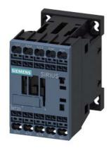
power contactor, AC-3 12 A, 5.5 kW / 400 V 1 NC, 24 V DC 0.7-1.25\* US, with varistor integrated, 3-pole Size S00, Spring-type terminal
