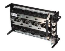
SIEMENS LOW VOLTAGE PL SERIES UNASSEMBLED LOAD CENTER. MAIN LUG INTERIOR WITH 24 1-INCH SPACES ALLOWING MAX 42 CIRCUITS. 3-PHASE 4-WIRE SYSTEM RATED 120/240V OR 120/208V (200A) 100KA INTERRUPT. SPECIAL FEATURES: COPPER BUS, INTERCHANGEABLE MAIN.
