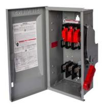
Siemens Low Voltage Circuit Protection Heavy Duty Safety Switches. Type: ENCLOSED, SAFETY SWITCH Std: UL V. Rating: 240V A. Rating: 60A Wattage: 4W No. Of Poles: 3P F. Rating: 60Hz Action: SINGLE THROW Material: 304SS Enclosure: TYPE 3R. 2-3 point mounting holes. O. Cycles: 10000 O. Temperature: (-20F-120F) AMBIENT TEMPERATURE Environmental Conditions: OUTDOOR
