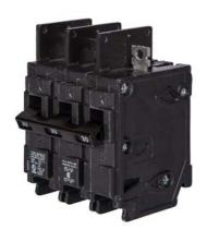
Siemens Low Voltage Molded Case Circuit Breakers General Purpose MCCBs are Circuit Protection Molded Case Circuit Breakers. 3-Pole Common-Trip circuit breaker type BQ. Rated 240 V (090A) (AIR 10 kA). Special features: Load side lugs are included.
