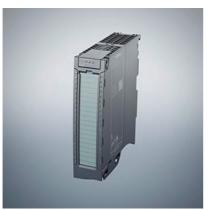
SIMATIC S7-1500, digital output module DQ 16x 230 V AC/2A ST; Relay 16 channels in groups of 2; 4 A per group; switching cycle counter for integrated relay, diagnostics; substitute value: the module supports the safety-oriented shutdown of load groups up to SILCL1 according to EN 62061:2005 + A2:2015, and Category 2 / PL c according to EN ISO 13849-1:2015. front connector (screw terminals or push-in) to be ordered separately
