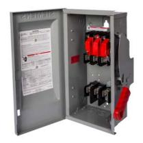
Siemens Low Voltage Circuit Protection Heavy Duty Safety Switch. 3-Pole 3-Fuse and solid neutral Fused in a type 1 enclosure (indoor). Rated 240VAC (200A).
