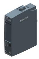
SIMATIC ET 200SP, Digital output module, DQ 8x 24V DC/0,5A Sink Basic, Sink output (NPN, M-switching), Packing unit: 1 piece, fits to BUtype A0, Colour Code CC01, substitute value output, module diagnostics for: supply voltage
