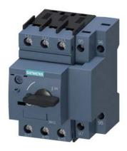
Circuit breaker size S00 for motor protection, CLASS 10 with overload relay function A-release 7...10 A N release 130 A screw terminal Standard switching capacity
