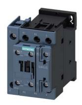
Contactor, 2NO + 2NC, AC-3, 11 kW, 110 V AC, 50 Hz, 120 V, 60Hz, 4-pole, 2NO + 2NC, Size S0, Screw terminal 1 NO + 1 NC integrated
