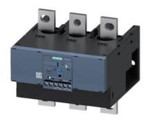
Overload relay 160...630 A for motor protection Size S10/S12, Class 10E Contactor mounting/stand-alone installation Main circuit: busbar connection Auxiliary circuit: Screw terminal Manual-Automatic-Reset
