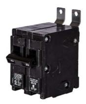
Siemens Low Voltage Molded Case Circuit Breakers Panelboard Mounting 240V Circuit Breakers - Type BL, 2-Pole, 120/240VAC are Circuit Protection Molded Case Circuit Breakers. Type: HBL Application: Electrical Distribution Standard: UL 489 Voltage Rating: 120/240V Amperage Rating: 100A Trip Range: Thermal Magnetic Interrupt Rating: 65 AIC Number Of Poles: 2P
