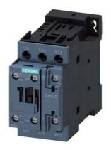
power contactor, AC-3 9 A, 4 kW / 400 V 1 NO + 1 NC, 24 V DC with plugged-in diode combination, 3-pole Size S0, screw terminal
