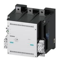
Contactor, Size 14, 3-pole, AC-3, 335kW, 400/380 V (690 V) Auxiliary switch 44 (4NO+4NC) AC operation 110...132 V AC 50/60 Hz
