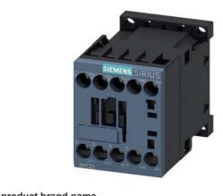
power contactor, AC-3 9 A, 4 kW / 400 V 1 NO, 24 V DC 0.7-1.25\* US, with diode integrated, 3-pole, size S00, screw terminal suitable for PLC outputs not expandable with auxiliary switch
