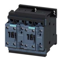
Reversing contactor assembly AC-3,11 kW/400 V,AC24V,50/60 Hz 3-pole, Size S0 screw terminal electrical and mechanical Interlock 2 NO integrated
