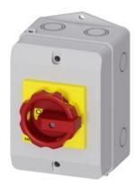
SENTRON, Switch disconnector 3LD, emergency switching-off switch, 3-pole, Iu: 25 A, operating power / at AC-23 A 400 V: 9.5 kW, Molded plastic encapsulation for inch cable gland, rotary operating mechanism, red/yellow
