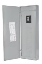
SIEMENS LOW VOLTAGE PL SERIES LOAD CENTER. FACTORY INSTALLED MAIN BREAKER WITH 42 1-INCH SPACES ALLOWING MAX 60 CIRCUITS. 3-PHASE 4-WIRE SYSTEM RATED 120/240V OR 120/208V (200A) 22KA INTERRUPT. SPECIAL FEATURES: COPPER BUS, INTERCHANGEABLE MAIN, GRAY TRIM, NEMA TYPE3R ENCLOSURE FOR OUTDOOR USE.
