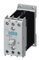
solid-state contactor 3-phase 3RF2 AC 51 / 22 A / 40  $^{\circ}\text{C}$  48-600 V / 4-30 V DC 2-phase controlled screw terminal blocking voltage 1200 V
