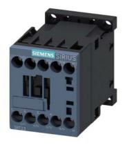
Contactor, AC-1, 22 A/400 V/40  $^{\circ}\text{C}$  , S00, 4-pole, 220 V AC/50 Hz, 240 V/60 Hz, screw terminal
