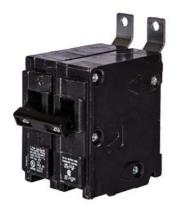
Siemens Low Voltage Molded Case Circuit Breakers Panelboard Mounting 240V Circuit Breakers - Type BL, 2-Pole, 120/240VAC are Circuit Protection Molded Case Circuit Breakers. Type: BLH Application: Electrical Distribution Standard: UL 489 Voltage Rating: 120/240V Amperage Rating: 100A Trip Range: Thermal Magnetic Interrupt Rating: 22 AIC Number Of Poles: 2P
