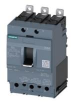
molded case switch 3VA4 UL frame 125 max. sh-circ breaking capacity 65kA @ 480 V 3-pole, line protection MCS110, In=100A without overload protection self-protection li=16 x In clamp connection
