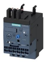
Overload relay 1...4 A Electronic For motor protection Size S00, Class 10E Contactor mounting Main circuit: Spring-type terminal Auxiliary circuit: Spring-type terminal Manual-Automatic-Reset
