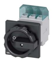
SENTRON, Switch disconnector 3LD, main switch, 3-pole, lu: 32 A, Operating power / at AC-23 A at 400 V: 11.5 kW, front-mounted, rotary operating mechanism, black, central mounting 22.5 mm of the handle
