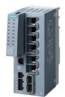
SCALANCE XC206-2SFP managed Layer 2 IE switch; IEC 62443-4-2 certified; 6x 10/100 Mbps RJ45 ports; 2x 100/1000 Mbps SFP; 1x console port; diagnostics LED; redundant power supply; temp. range -40 °C to +70 °C; mounting: DIN rail/S7 mounting rail/wall Office redundancy functions features (RSTP, VLAN,...); PROFINET IO device; Ethernet/IP-compliant; C-plug slot;
