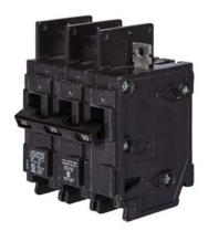
Siemens Low Voltage Molded Case Circuit Breakers General Purpose MCCBs are Circuit Protection Molded Case Circuit Breakers. 3-Pole Common-Trip circuit breaker type BQ. Rated 240 V (100 A) (AIR 10 kA). Special features: Load side lugs are included.
