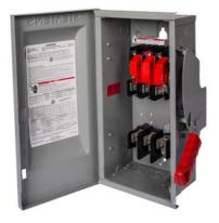
Siemens Low Voltage Circuit Protection Heavy Duty Safety Switches. Type: ENCLOSED, SAFETY SWITCH Std: CUL V. Rating: 600V A. Rating: 200A Wattage: 6W No. Of Poles: 6P F. Rating: 60Hz Action: SINGLE THROW Material: 304SS Enclosure: TYPE 3R/12. 2-3 point mounting holes. Insulation: YES O. Cycles: 8000 O. Temperature: (-20F-120F) AMBIENT TEMPERATURE Environmental Conditions: OUTDOOR/INDUSTRIAL
