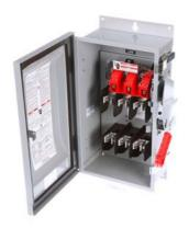
Siemens Low Voltage Circuit Protection Heavy Duty Safety Switches. Type: ENCLOSED, SAFETY SWITCH Std: UL V. Rating: 600V A. Rating: 30 A Wattage: 3W No. Of Poles: 3P F. Rating: 60Hz Action: SINGLE THROW Material: 304SS Enclosure: TYPE 12. 2-3 point mounting holes. Insulation: YES O. Cycles: 10000 O. Temperature: (-20F-120F) AMBIENT TEMPERATURE Environmental Conditions: INDUSTRIAL
