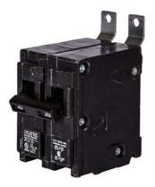
Siemens Low Voltage Molded Case Circuit Breakers Panelboard Mounting 240V Circuit Breakers - Type BL, 2-Pole, 120/240VAC are Circuit Protection Molded Case Circuit Breakers. Type: BL Application: Electrical Distribution Standard: UL 489 Voltage Rating: 120/240V Amperage Rating: 10A Trip Range: Thermal Magnetic Interrupt Rating: 22 AIC Number Of Poles: 2P
