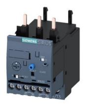
Overload relay 1...4 A Electronic For motor protection Size S0, Class 10E Contactor mounting Main circuit: Screw Auxiliary circuit: Screw Manual-Automatic-Reset
