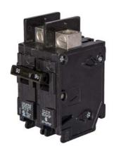
Siemens Low Voltage Molded Case Circuit Breakers General Purpose MCCBs - Type BQ, 2-Pole, 120/240VAC are Circuit Protection Molded Case Circuit Breakers. 2-Pole Common-Trip circuit breaker type BQ. Rated 120/240V (100 A) (AIR 10 kA). Special features: Load side lugs are included.
