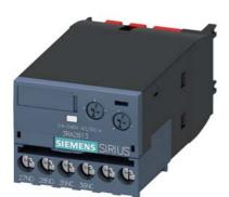
Solid-state time-delayed auxiliary switch ON delay Relay 1 NC + 1 NO 24...240 V AC/DC Time range 0.05...100 s Can be snapped on at the front For 3RT2 S00-S3 contactors and 3RH2 S00 contactor relays Screw terminal Varistor for attenuation of the contactor coils integrated
