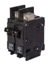
Siemens Low Voltage Molded Case Circuit Breakers General Purpose MCCBs - Type BQ, 2-Pole, 120/240VAC are Circuit Protection Molded Case Circuit Breakers. 2-Pole Common-Trip circuit breaker type BQ. Rated 120/240V (035A) (AIR 10 kA). Special features: line side lugs included. Note: Load side lugs are included.
