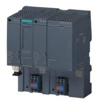
SIMATIC PN/PN Coupler for deterministic data exchange between max.4 PN-Controller per subnet, also from subnet to subnet, PROFIsafe data exchange, I/O-, MSI-, MSO- and data record communication, redundant power supply, PN-connection via SIMATIC BusAdapter (BA), delivery w/o BusAdapter
