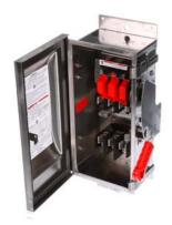
Siemens Low Voltage Circuit Protection Heavy Duty Safety Switches. Type: ENCLOSED, SAFETY SWITCH Std: UL V. Rating: 600V A. Rating: 30 A Wattage: 3W No. Of Poles: 3P F. Rating: 60Hz Action: SINGLE THROW Material: SS Enclosure: TYPE 4X. 2-3 point mounting holes. Insulation: YES O. Cycles: 10000 O. Temperature: (-20F-120F) AMBIENT TEMPERATURE Environmental Conditions: INDUSTRIAL CORROSIVE RESISTANCE
