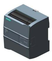
SIMATIC S7-1200, CPU 1211C, compact CPU, DC/DC/relay, onboard I/O: 6 DI 24 V DC; 4 DO relay 2A; 2 AI 0-10 V DC, Power supply: DC 20.4-28.8V DC, Program/data memory 50 KB
