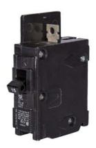
Siemens Low Voltage Molded Case Circuit Breakers General Purpose MCCBs are Circuit Protection Molded Case Circuit Breakers. 1-Pole circuit breaker type BQ. Rated 120V (020A) (AIR 10 kA). Special features: Load side lugs are included.
