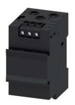
Current/voltage measuring module V2; Set current 0.3 ... 4 A, Voltage measurement up to 690 V, Overall width 45 mm, Straight-through transformer, basic unit required pro V PB, pro V MR, pro V PN or pro V EIP
