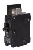
Siemens Low Voltage Molded Case Circuit Breakers General Purpose MCCBs are Circuit Protection Molded Case Circuit Breakers. 1-Pole circuit breaker type BQ. Rated 120V (020A) (AIR 10 kA). Special features: line side lugs included. Note: Load side lugs are included.
