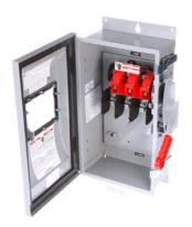
Siemens Low Voltage Circuit Protection Heavy Duty Safety Switches. Type: ENCLOSED, SAFETY SWITCH Std: UL V. Rating: 600V A. Rating: 200A Wattage: 2W No. Of Poles: 3P F. Rating: 60Hz Action: SINGLE THROW Material: 304SS Enclosure: TYPE 12. 2-3 point mounting holes. Insulation: YES O. Cycles: 8000 O. Temperature: (-20F-120F) AMBIENT TEMPERATURE Environmental Conditions: INDUSTRIAL
