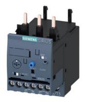
Overload relay 0.1...0.4 A Electronic For motor protection Size S0, Class 10E Contactor mounting Main circuit: Screw Auxiliary circuit: Screw Manual-Automatic-Reset
