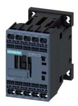
power contactor, AC-3 7 A, 3 kW / 400 V 1 NC, 24 V DC 0.7-1.25\* US, suppressor diode integrated, 3-pole, size S00, spring-type terminal not expandable with auxiliary switch
