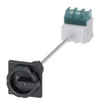
SENTRON, Switch disconnector 3LD, main switch, 3-pole, lu: 63 A, Operating power / at AC-23 A at 400 V: 22 kW, floor mounting with door coupling, rotary operating mechanism, black, central mounting 22.5 mm of the handle
