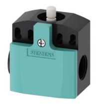
position switch plastic enclosure 50 mm, device connection 2 x (M20 x 1.5) 1 NO/1 NC integrated (not replaceable) quick-action contacts, rounded plunger
