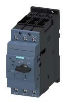
Circuit breaker size S2 for motor protection, CLASS 10 A-release 18...25 A N-release 325 A Screw terminal Standard switching capacity
