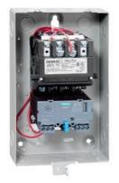
Non-reversing motor starter, Size 00, Three phase full voltage, Solid-state overload relay, OLR amp range 3-12A, 110V 50Hz / 120V 60Hz coil, Noncombination type, Enclosure type 1, Indoor general purpose use, Standard width enclosure
